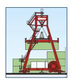
Transtainers are the cranes operating on big blocks of containers on the Yard or on Rail Terminal for handling containers from the ground to vehicles, trucks, or flat-cars of trains.
