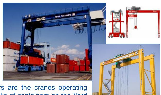
Transtainers are the cranes operating on big blocks of containers on the Yard or on Rail Terminal for handling containers from the ground to vehicles, trucks, or flat-cars of trains.
