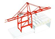
The Portainers (known also gantry cranes, ship-to-shore cranes) are operating from the Dock to load and unload the ships
