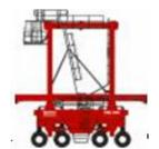
A **Straddle Carrier** is an handling device in use in some port terminals for moving and stacking standard containers.
